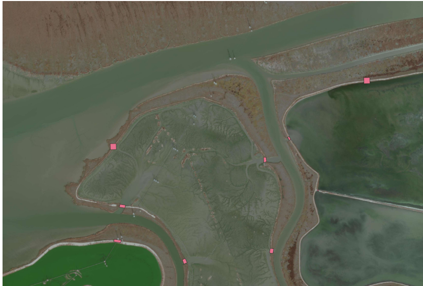
Figure 15. Example of identified possible levee breaches in South Bay. The pink boxes represent the breaching locations. The middle of each breach was used in combination with a 1000-foot wide circle to adjust the model bathymetry and weir. The depth is based on mean lower low water (MLLW).
